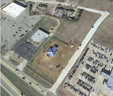
Hayter Engineering provided a preliminary and final plat for 5.532 acres for Paris SMPC Addition 322. In the photo above the new roadway adjoins Loop 286 by the ORR Honda Dealership and joins Levi Lane in the new development. The street is 39' wide x 7" thick concrete and approximately 1,100 linear feet in length.
